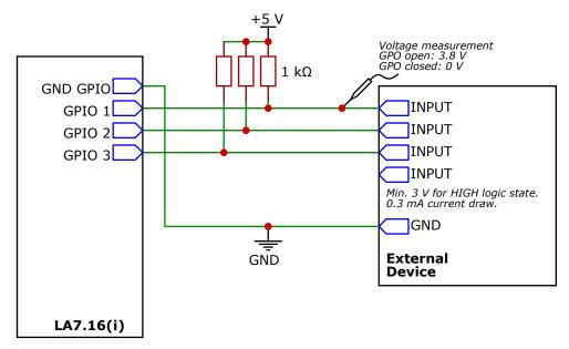
When the GPO is  ${f closed}$ , the GPI of the external device is set to  ${f LOW}$  logic state.
