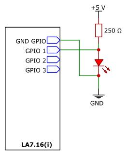
When the GPO is **closed**, the LED is **turned off** (the LED is short-circuited by the contact relay). When the GPO is **open**, the LED is **turned on**.
