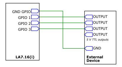
The TTL output of the external device can switch between +5 V and 0 V potentials, and is directly connected to the GPI port.
